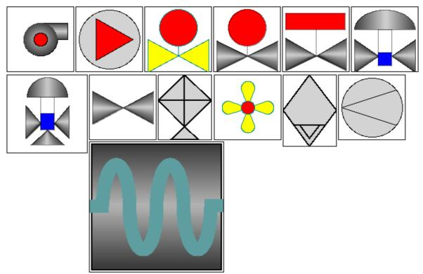
Fig.1. Elements representing technological devices from left to right and top to bottom: "Compressor", "Compressor 1", "Bolt", "Crane", "Ball crane", "Crane and position", "Three-positioned crane", "Valve" "Cooler", "Cooler", "Separator", "Diaphragma", "Zmejev hor".
