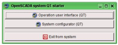
Fig.2. The dialog window of the "Starter".
