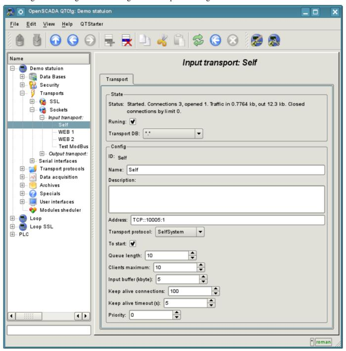
Fig. 1. Configuration dialog of the incoming socket.
