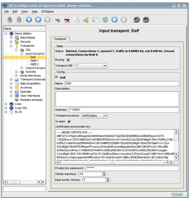
Fig. 1. Configuration dialog of the incoming SSL-transport.
