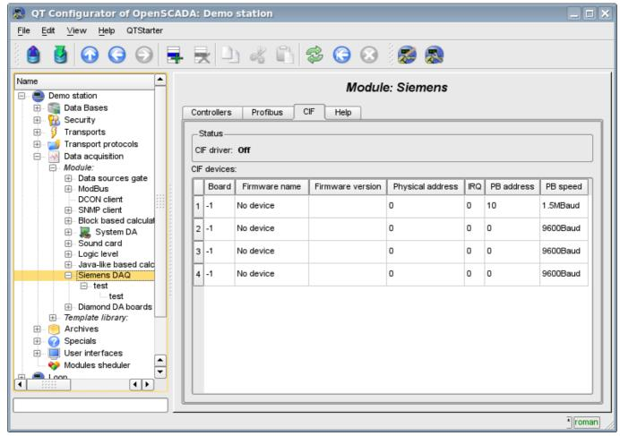
Fig.1. Configuration tab of CIF-boards.
