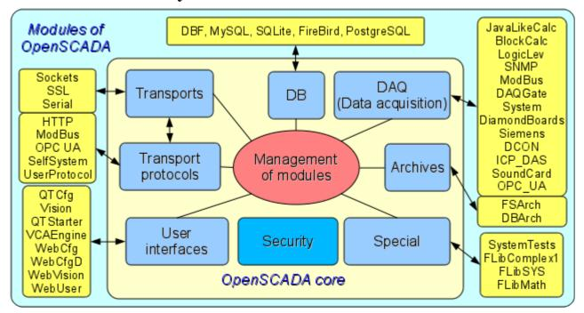
Fig. 1. The block scheme of OpenSCADA system
