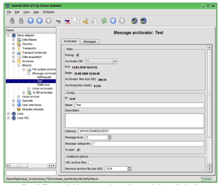
Fig. 4.6h. The main tab of the messages archiver configuration of subsystem "Archives".
