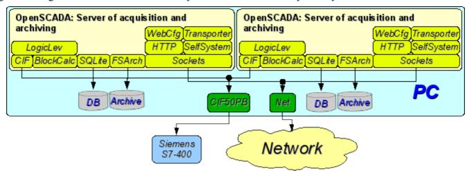
Fig. 3.3. The duplicated server connection on one server.
