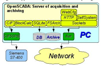
Fig. 3.1. Simple server connection.
