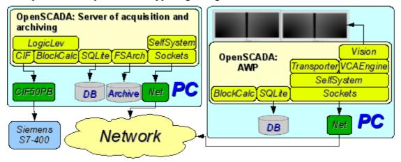
*Fig. 3.5. The automated workplace (place of the manager/operator).*
