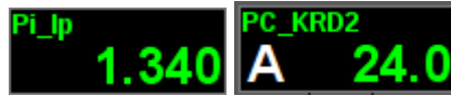
Fig.1. "Analog show" widget in the development and runtime modes (left to right).
