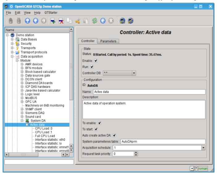
Fig.1. Tab of configuration of the controller.
