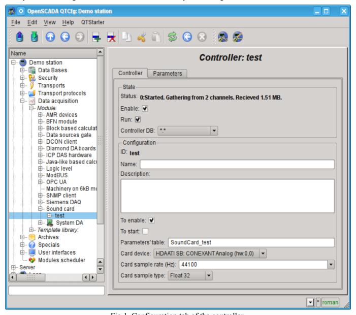
Fig. 1. Configuration tab of the controller.
