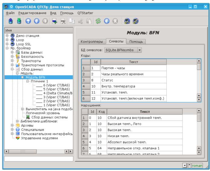
Fig. 1. Configuration tab of signals and alarms symbols.
