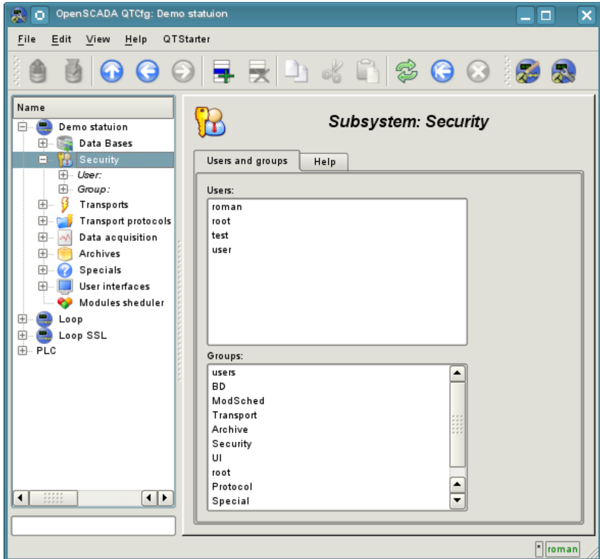
Fig. 4.2a. Tab "Users and Groups" of the root page of the subsystem "Security".
