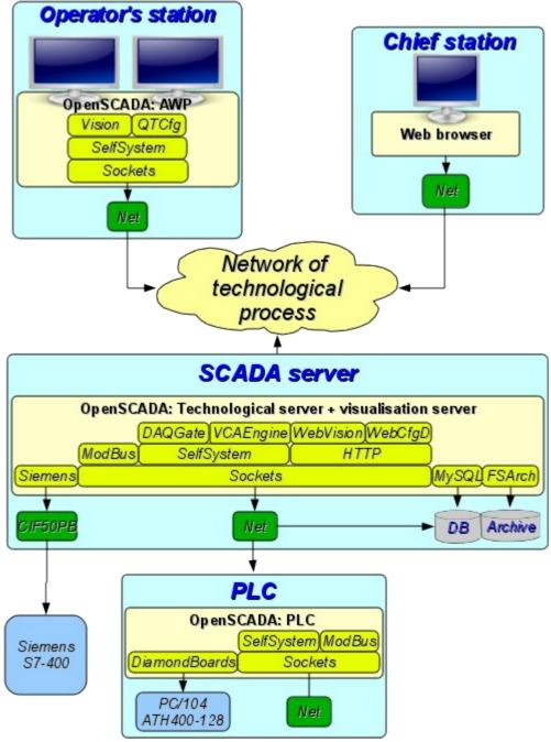
Fig. 1. OpenSCADA system's roles
