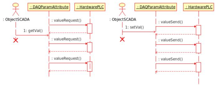
Fig. 3. Diagram of interaction sequence with asynchronous requests.
