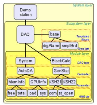
Fig. 1. The subsystem's "Data acquisition" scheme.
