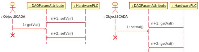
Fig. 5. Diagram of interaction sequence with the passive working mode.
