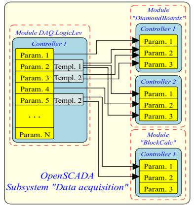
Fig. 7. The mechanism of the "Logic level" on the example of LogicLev module.
