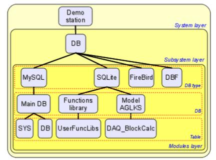
Fig. 4.1a. The hierarchical structure of "DB" subsystem.
