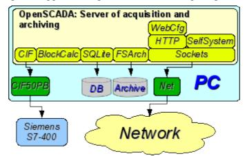
Fig. 3.1. Simple server connection.
