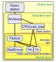
Fig. 4.6a. The hierarchical structure of subsystem "Archives"
