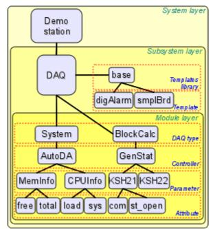
Fig. 4.5a. The hierarchical structure of subsystem "Data acquisition".
