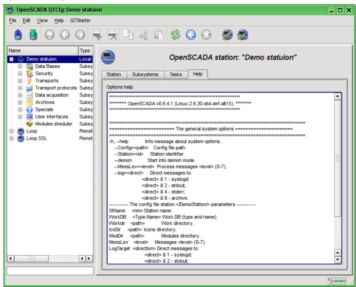
Fig. 4.10a. The "Help" tab of the OpenSCADA component.
