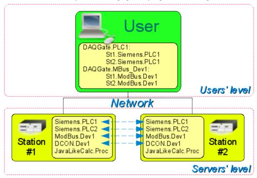
Fig.1. Horizontal and vertical redundancy.
